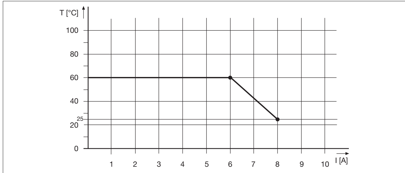
Derating diagram (PSSu E F BSW): Permitted ambient temperature T dependent on load current I
